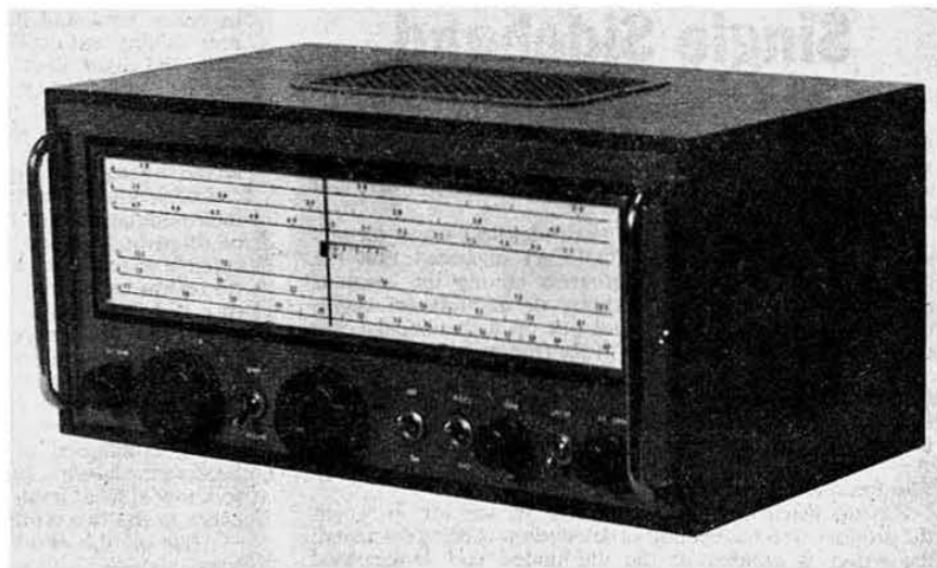
A three-quarter view of the home-built communications receiver in its wooden cabinet. The controls, from left to right, are r.f. gain, bandswitch, send/receive switch, tuning, main on/off, a.g.c./b.f.o. switch, b.f.o. tuning, noise limiter on/off and a.f. gain.
