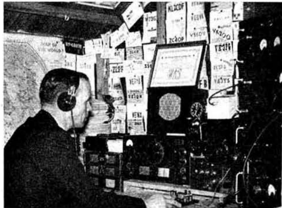
Art Trigell (G3JAF) operates from Lymington in Hampshire. The home-built transmitter uses a pair of 807s with clamp modulation, while the receiver is an HRO modified for 6BA6s in the r.f. stages and preceded by an RF24 Unit on 10 and 15 metres. The aerial is a two-band quad 43 ft. in the air. Art has 182 countries confirmed from 204 worked, WAZ and WAS and is only one confirmation short of EDXC.
