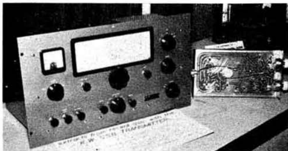
The new K.W. Electronics filter-type single sideband transmitter which uses printed circuits. A typical sub-assembly is shown on the right of the picture. (Photo by G2AHL.)
