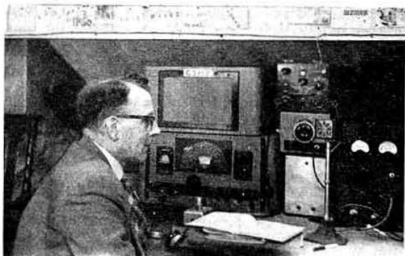
G3JLF of Blackpool uses an RME45 receiver and a Minimitter transmitter with a half-size G5RV-type aerial and indoor dipoles for 21 and 28 Mc/s.
